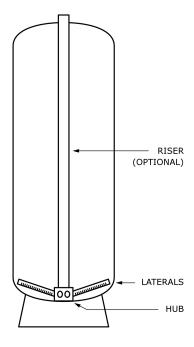
SWT's Water's Edge Distributor System Kits for Top Mount Tanks are fabricated from non-corrosive FDA and NSF approved materials for use in softeners, deionizers, carbon filters, sediment filters, iron filters, and multimedia filters. They are designed for all top mount control valves with a 1-1/2 inch center riser port.
